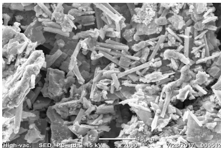
Figure 5. SEM image of SnO 2 nanorod annealing at 600°C
