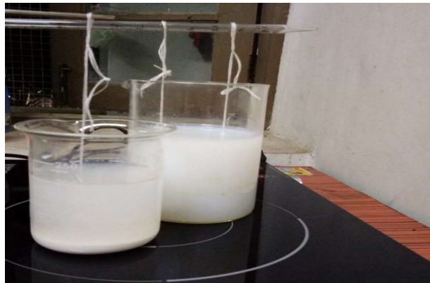
Figure 3. SnO 2 seed layer coated FTO glasses immersed into the aqueous solution
